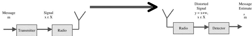
Fig. 1. Signal plus noise without multipath.
